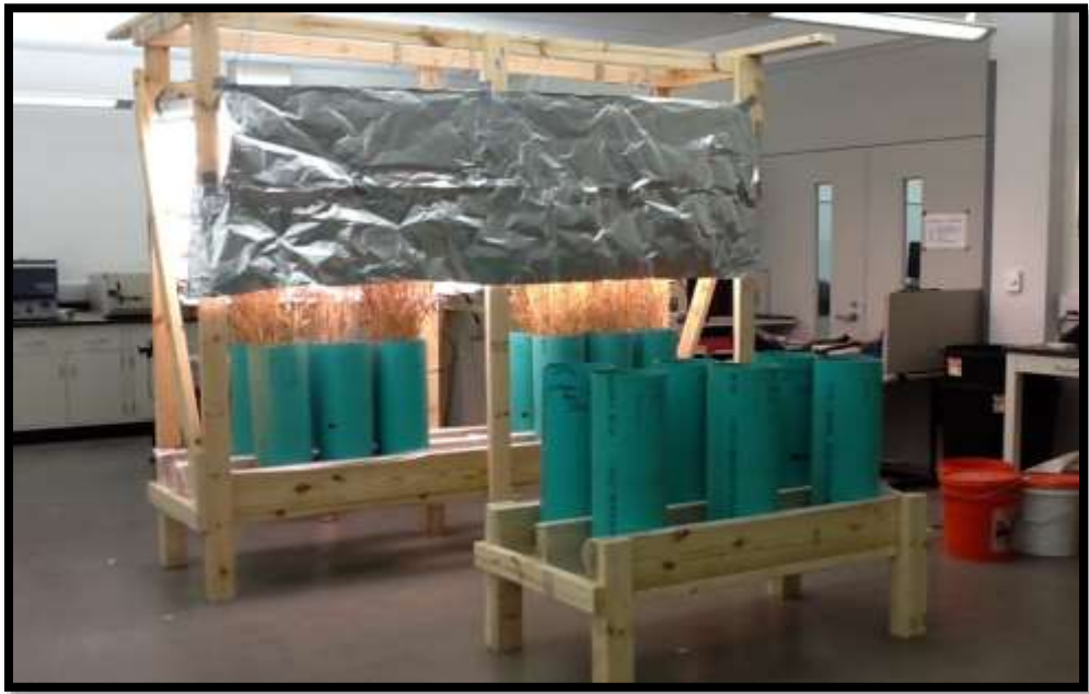
Figure 6. Column Framework and Support
