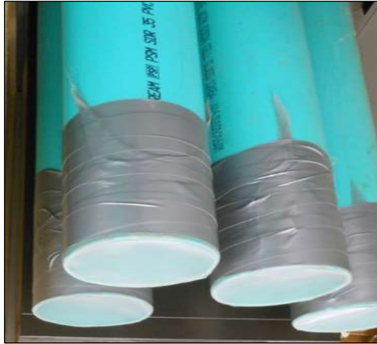
Figure 5. Columns with Fibreglass Window Screen Attached to the Bottom
